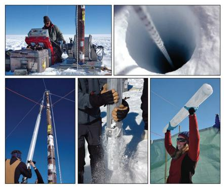
Figure 1. Ice Core Sampling.
